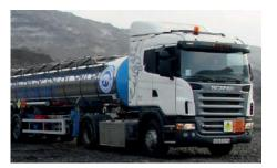
Tank semi-trailer ADR 17-1 designed for transportation of ammonium nitrate solution. Total weight of the transported solution – 22,7 tons. Tank has heat proof, liquid heating system and could be equipped with a pump. Pump drive could be hydraulic or electric. The tank has 3 hatches with diameters of 500 mm.h
