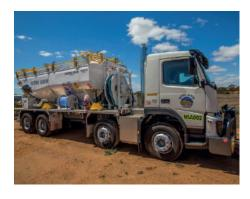
**Mixing and charging truck MSZ-20UT** is intended both for transportation of explosive's components and manufacturing of the following types of commercial explosives:
