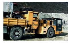
**Underground charging unit MP-1600** is mounted on a multipurpose vehicle PAUS, but could also be installed on an analogous chassis.
