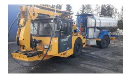
Underground mixing-and-charging truck 'MSZP-4' Mixing-and-charging truck 'MSZP-4' is designed for loading vertical and deviated boreholes with a diameter of 60 mm to 120 mm, a depth of 40 m and an angle of inclination to the horizon of 0 ° to 90 ° during stoping and blasting operations applying emulsion explosive 'Sibirit'. For charging at ambient temperatures from +5 °C to +45 °C.
